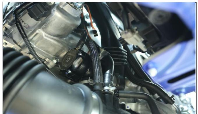
4) Remove the diverter vacuum hose from the car and replace with the hose supplied with the GFB Respons TMS kit.
